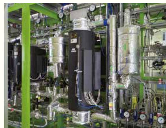
Demonstration of durability of zeolite catalyst with small pilot apparatus for olefin synthesis
